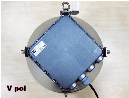
1 Remove Integra-W FODU with an antenna from mounting bracket. Default polarization is vertical.
