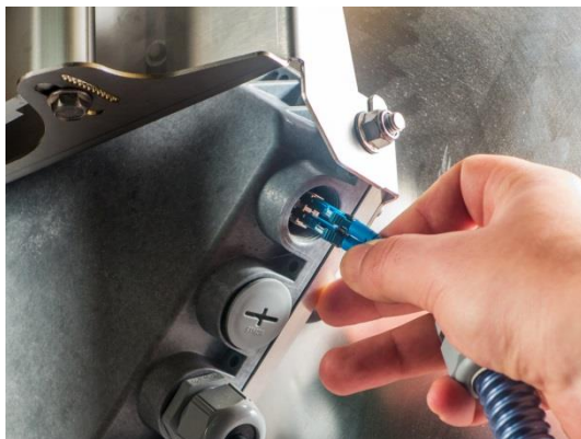
5 Connect LC connector to SFP module.
