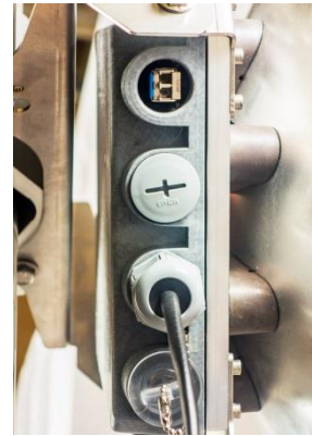
2 Unscrew the cap of the LAN-SFP port that will be used and install an SFP module.
