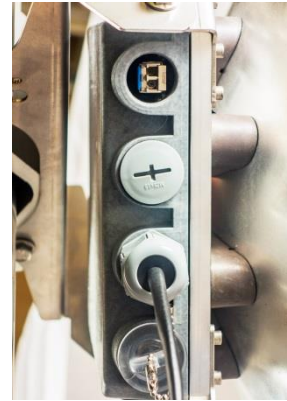
2 Unscrew the cap of the SFP port (LAN2 or LAN3) that will be used and install an SFP module.
