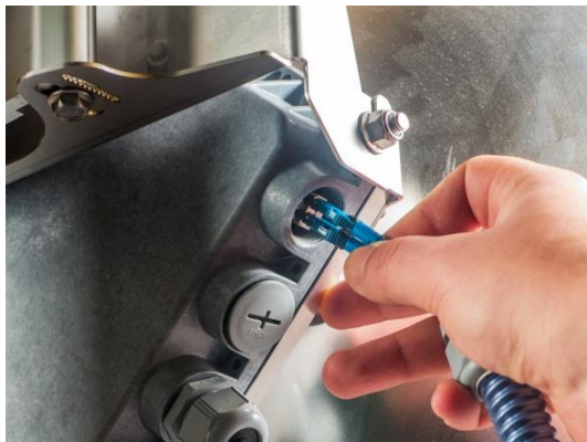
5 Connect LC connector to SFP module.
