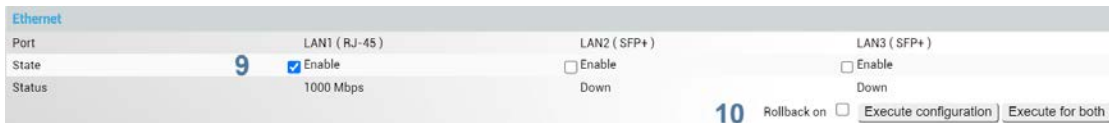
Figure 3-32 Ethernet section of ACAP and ACCP modes Main page in modify mode
