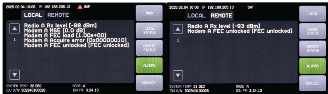
Figure 5-39 Alarm status display examples
