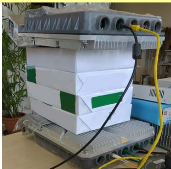
Figure 2-2 Example of Integra FODU link bench test with office paper packs
