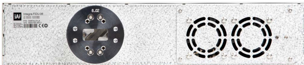
Figure 7-16 Antenna port on the back panel of Integra-FIDU/FIDU+ with diplexer
